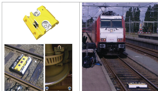
Slika 1. Sistem UVIS (Under Vehicle Inspection System) [7]
