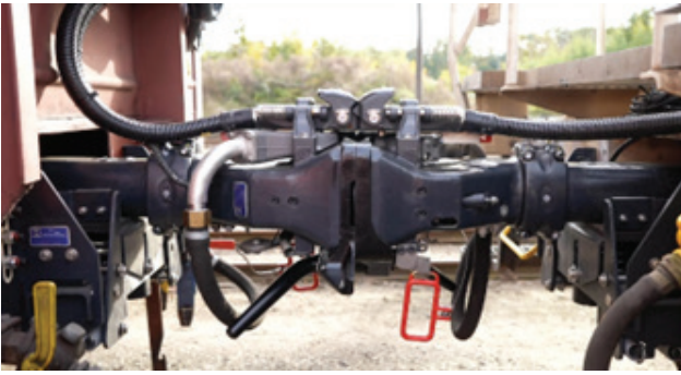
Figure 1: DAC Type Scharfenberg from Voith. Source: (Voith GmbH & Co. KGaA, 2022)
