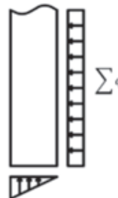
Figure 5. Elastostatic principle for a stable wall
