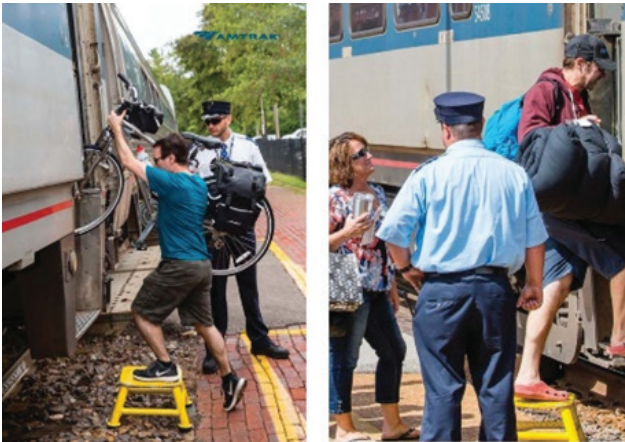
Figure 2. Inconsistency of the platform height with the entrance to the vehicle ( https://www.amtrak.com/content/dam/projects/dotcom/english/public/documents/corporate/businessplanning/Amtrak-Five-Year-Service-Plans-FY18-FY23.pdf , 28.08.2023.)
