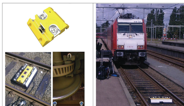
Slika 1. Sistem UVIS (Under Vehicle Inspection System) [7]
